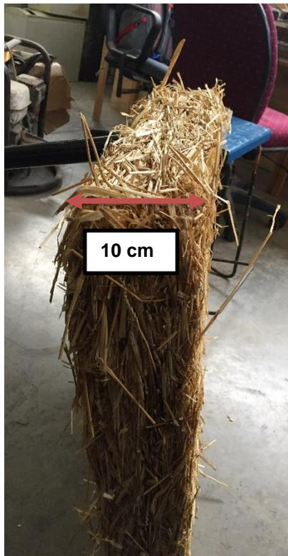
Figura 3-17: Espesor aislante "A" 100mm (70/30%).
