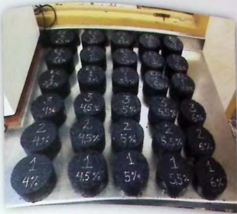
Figura 10.11: Probetas Marshall.
