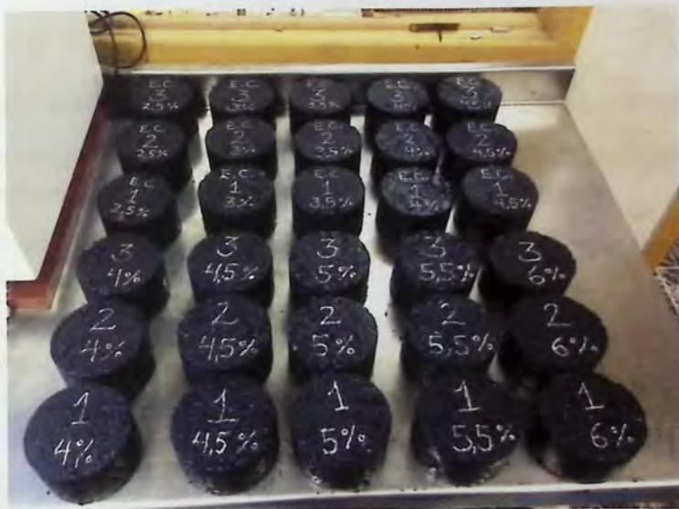
Figura 4.3: Probetas Marshall.
