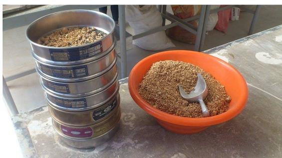
Figura 4.5 Serie tamices ASTM
