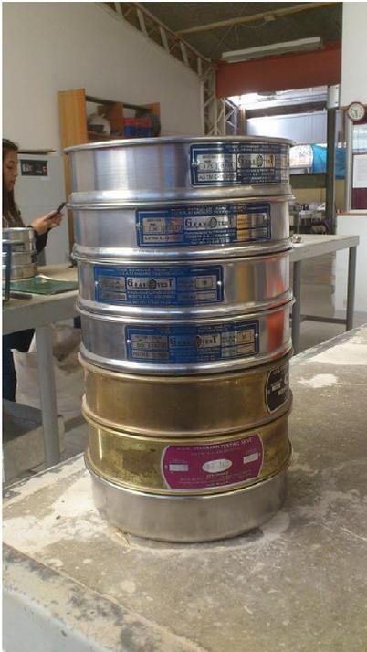
Figura 4.2: Serie Tamices ASTM
