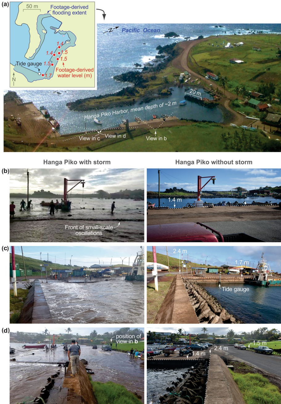
Fig. 7 Field survey results and visual effects of the May 5th, 2020, extreme sea-level event at Hanga Piko. a Aerial view of the Hanga Piko Harbor and water levels and inundation extents, as derived from video and photographic footage. b–d Comparisons of photographs taken at the same site with similar tide levels (0.2 m above MSL) during this event and calm conditions. The left panel of b is a video frame
