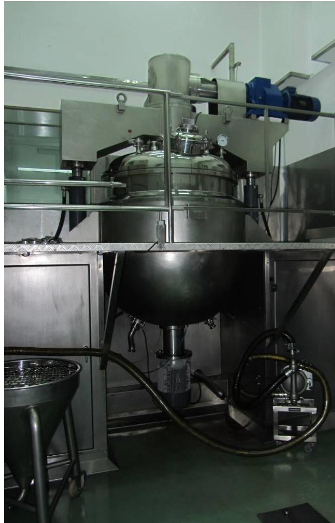
Figura N° 7: Reactor Naarden Triplex 1.000 L
