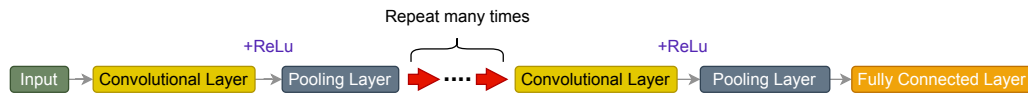
Figure 2.11: Scheme of a Convolutional Neural Network. Source: adapted from Becker et al. (2020)
