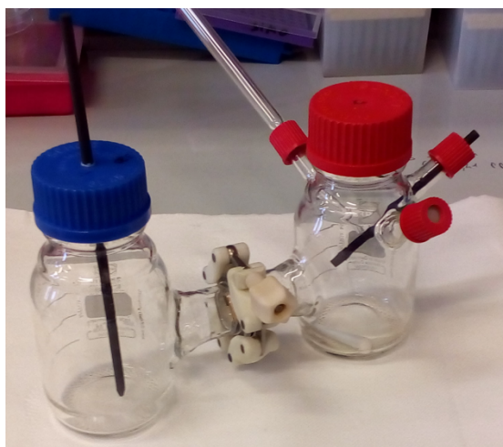
Figure 8. Two-chambers BES used in all the experiments.
