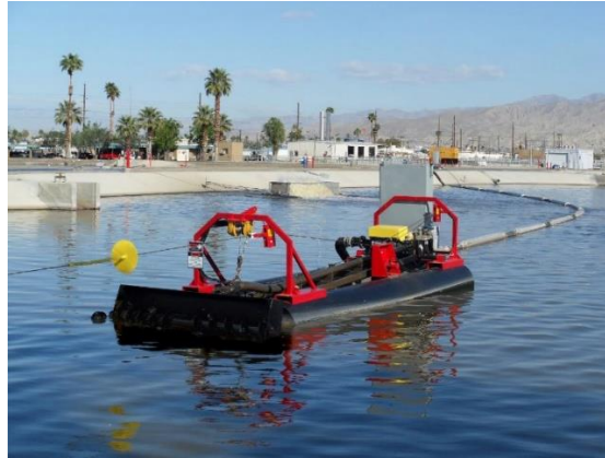
Figura 1.14: Draga Pit Hog. Mud Cat TM . mudcatdredge.com .
