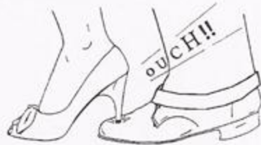
Fig 1b. The heel of the lady's shoe is exerting a point-loading of 1200 tonnes/m 2 .
