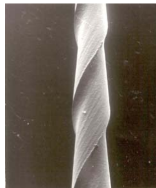
Fig.20: MEB Cuerpo de lima NiTi-TEE 4/25 80X
