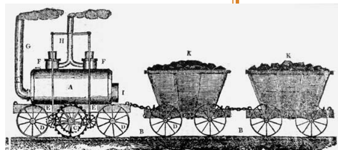
Description of the Plate. A. Boiler. B. Rail road. C. The propelling wheel, which is put in motion by the agency of steam, or any best mover. D. The carriage wheels. E. Connecting rods. F. Steam cylinders. G. Smoke chimney. H. Steam or discharging pipe. I. Fire place. K. Coal waggon, or carriages of any description.
