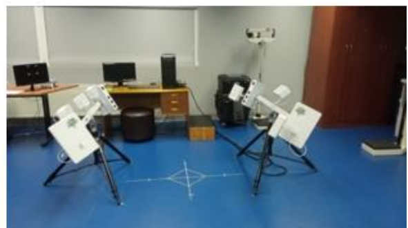
Figura 1 Scanner 3dMD, modelo cranial4 System
