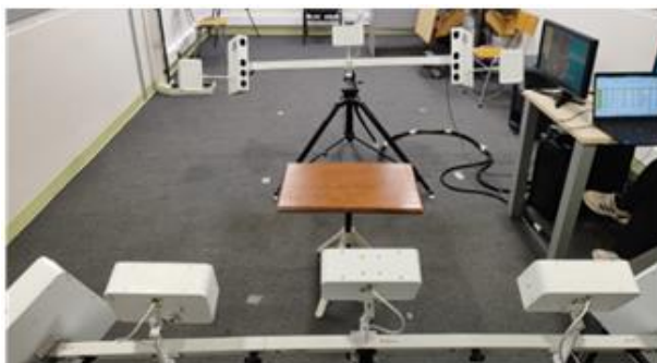
Figura 1 Scanner 3dMD, modelo cranial4 System
