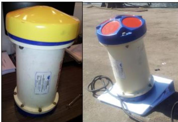
Figura 5-15: ADCP "Sentinel" de Teledyne RD Instrument
